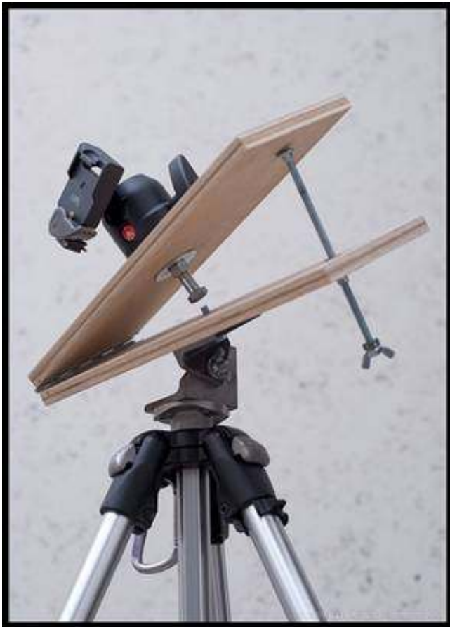
Above: a simple "Barn Door" camera mount for following the stars.
